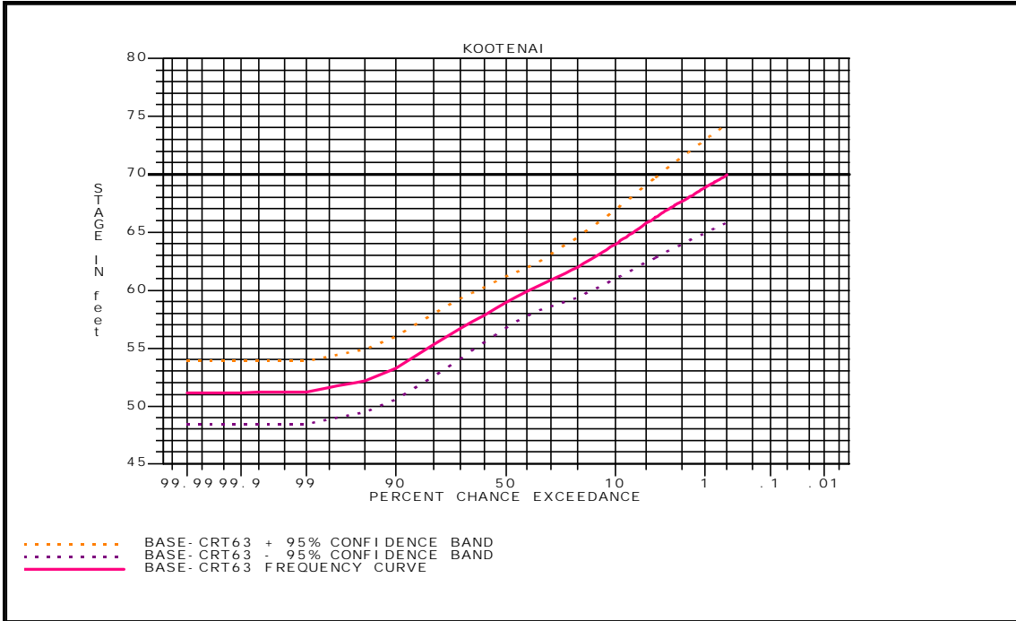
Figure 2-23. Frequency curve for Daily Peak Stage at Bonners Ferry with 95% Confidence Limits under BASE-CRT63.
