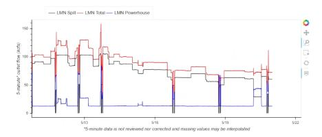
• The dips going below zero are to accommodate the barge loading and departure.
