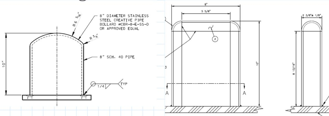
The image on the left are the Cascades Island bollards which will not be used. The bollards to the right will be used and were constructed at John Day North Fish Ladder.
