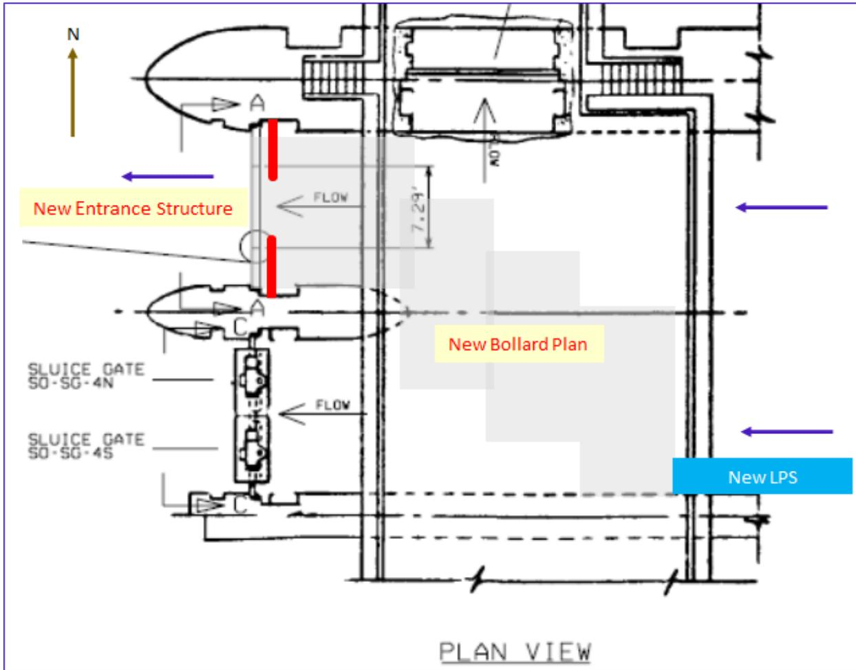
Figure 3-9. Plan Schematic of Paddle Bollard Arrangement at John Day North Fishladder.
