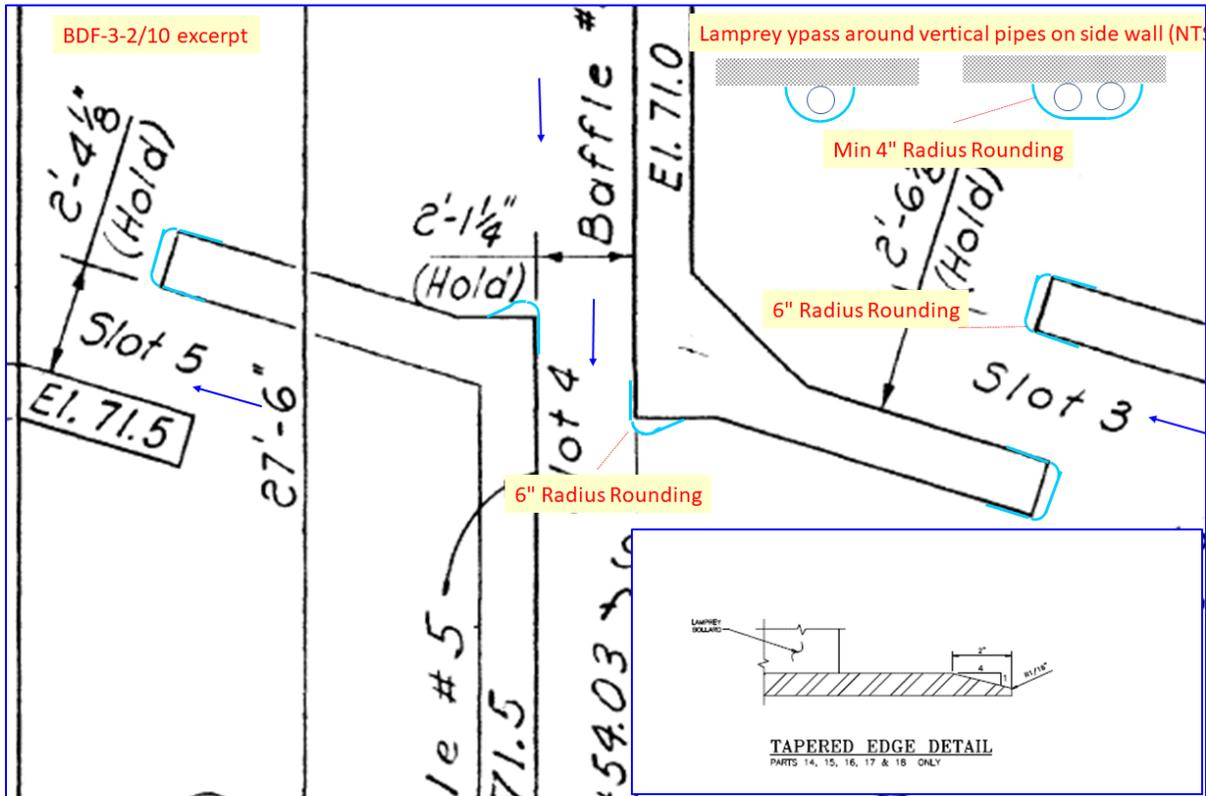
Figure 3-20. Bradford Island Exit Section Improvements: Plating into Exit Gate Opening, Plan
