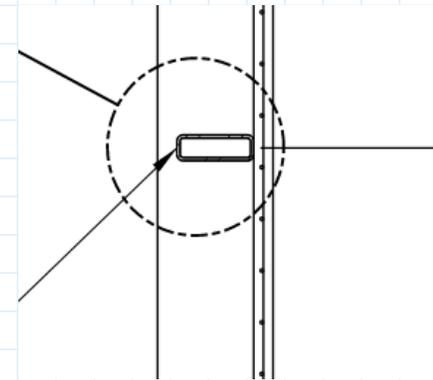
welding note: if forces are at right angles, weld force needs to be summed in x and y and sqrt.
