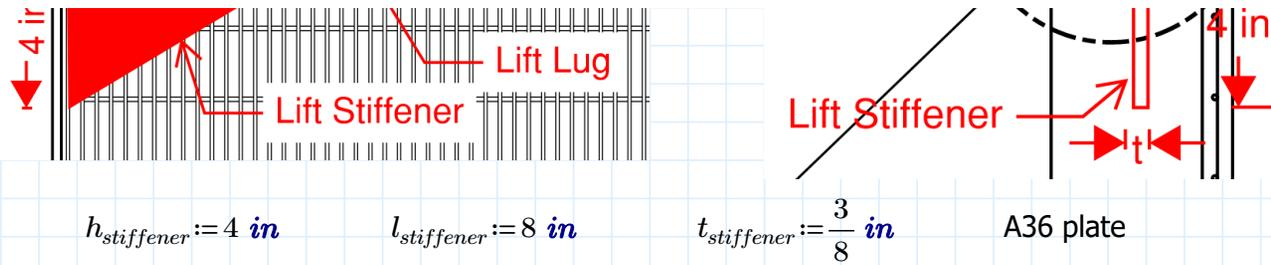
Weld size: 3/16" fillet weld, full length both sides to HSS member and end plate
