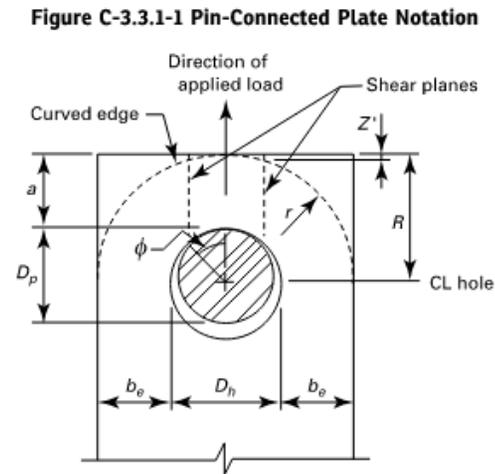
$$D_p := 1 \text{ in} \quad D_h := 1 \text{ in} + \frac{1}{8} \text{ in} = 1.125 \text{ in} \quad F_u := 58 \text{ ksi} \quad N_d := 2 \quad (\text{cat A lifter})$$
