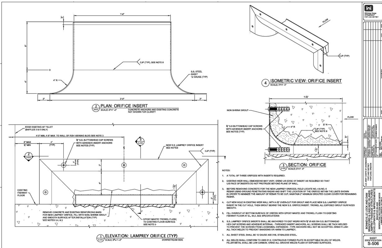
The orifices require some concrete excavation, followed by stainless steel plate insertions that are grouted in. The downstream face of the orifice is radiused 4-inches to provide means of attachment into the orifice. There is minimal radiusing on the upstream side, as the velocity is normally higher on the downstream side due to flow contraction. This is also done to reduce the overall flow increase in flow through the Serpentine exit section.
