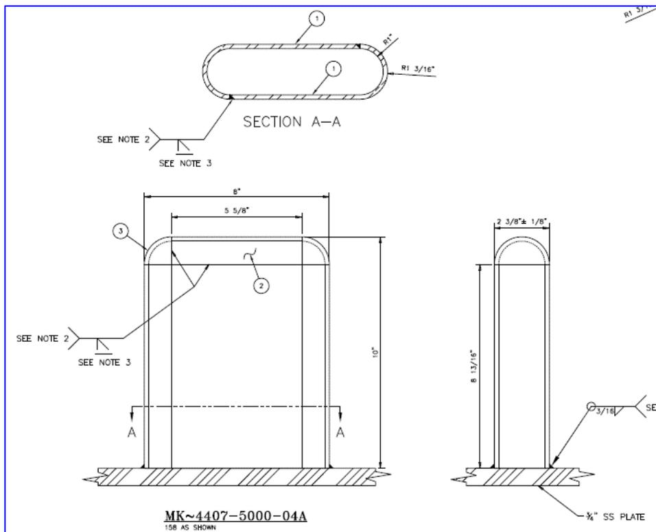
\*\* Excerpt Sheet SN101D, USACE (2015) John Day Lock and Dam North Fish Ladder Entrance Improvements Plans and Specifications, As-Constructed.
