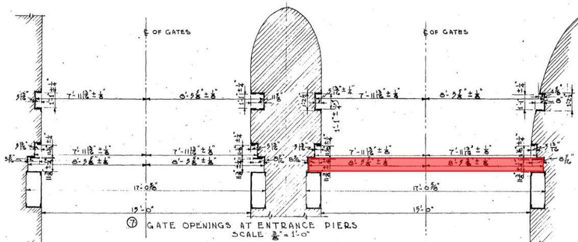
Figure 4-2: Plan View Showing the Entrance Slots and The Relevant Slot for the Weir
