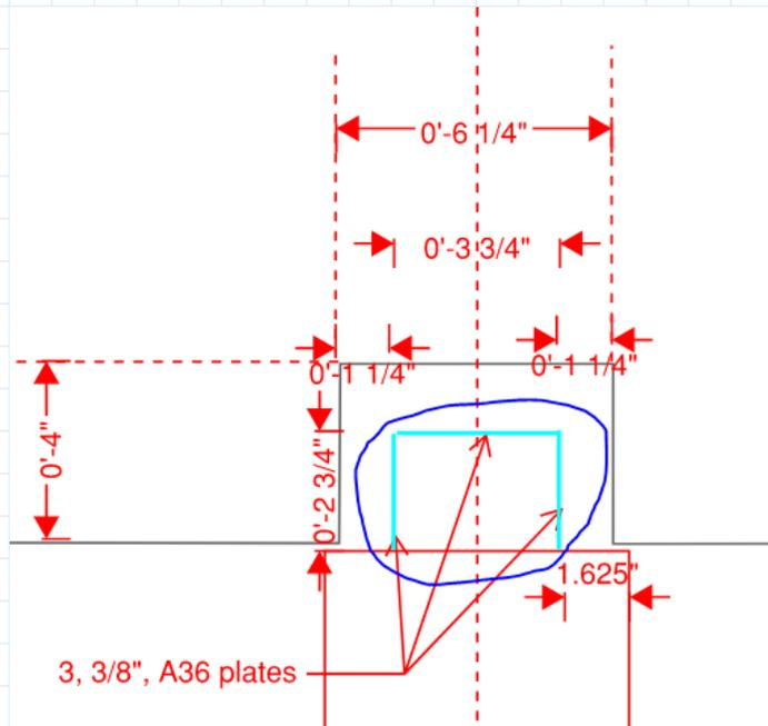
Geometry:  $F_y := 36 \text{ ksi}$  (A36 steel)  $h_{plate} := 1 \text{ ft}$  (design in per ft)
