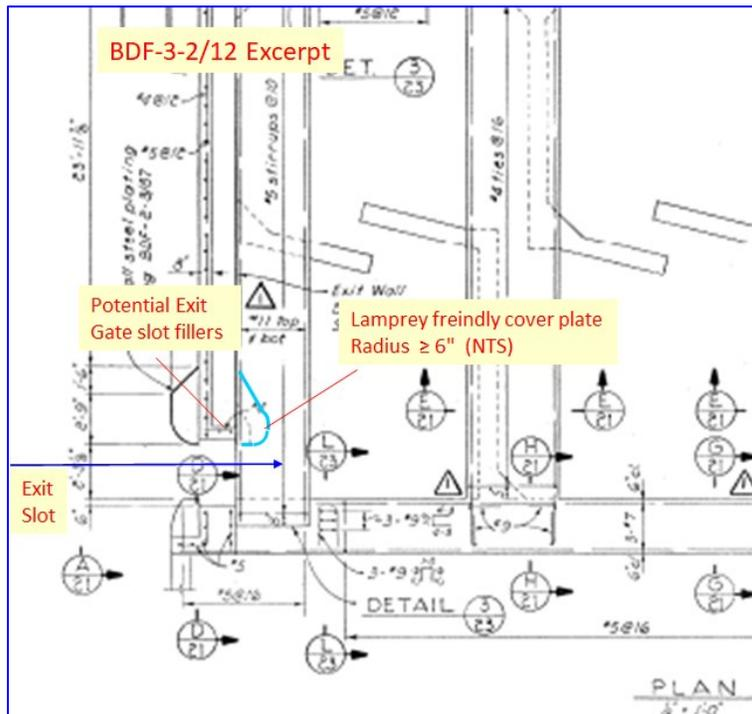
The plating material is up to the discretion of structural design. However, the plating material and means of anchoring will need to be non-metallic at the four PIT slots.
