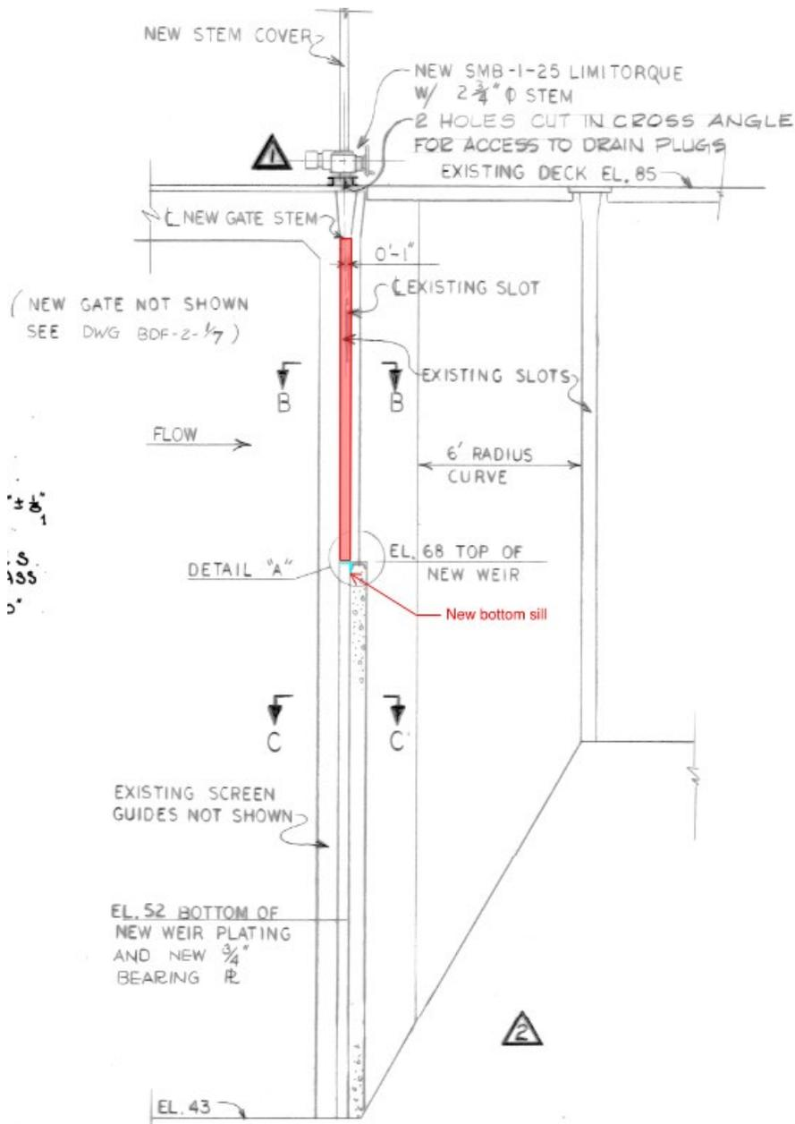
The rack will require a new sill at EL 68'. There is no need to use a trash rack below this elevation. The new sill will consist of a L8x8x1/2", welded to the existing concrete weir and its steel cap.
