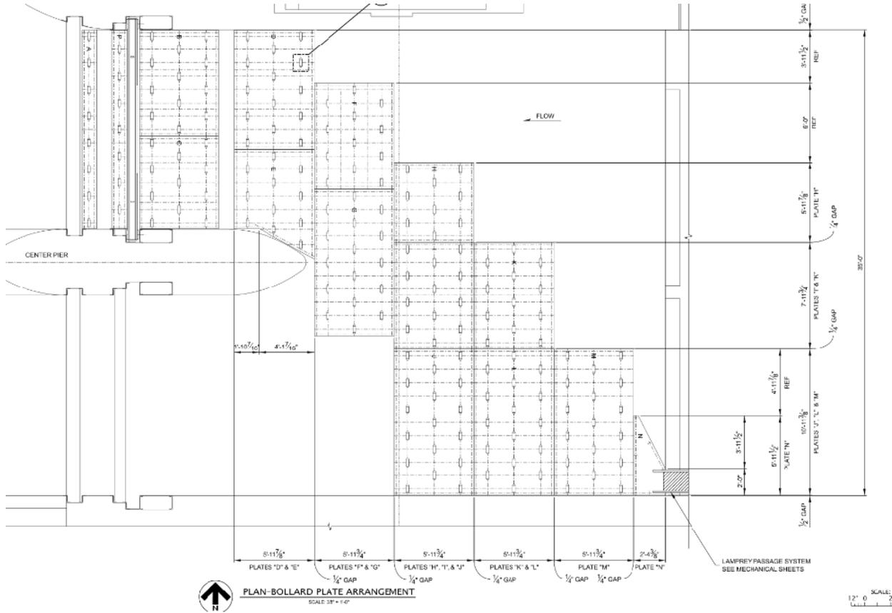
**Trash Rack:** A new trash rack is required to keep debris out of the LPS water supply pipe. The new rack will be positioned just upstream of the pipe and in an old sluice gate slot at the dam forebay. The trash rack slot is shown below on sheet BDF-2-1/4:
