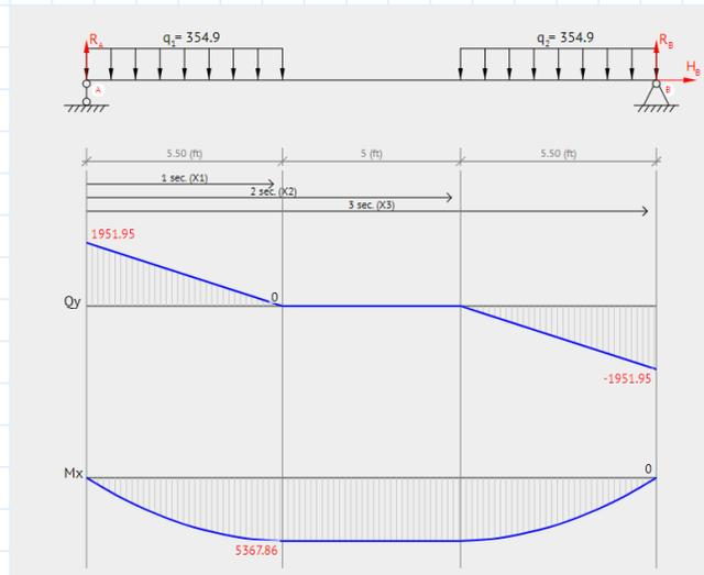
$$V_1 := 1951.95 \text{ lb} \quad M_1 := 5367.86 \text{ lb} \cdot \text{ft}$$
