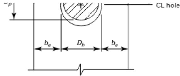
Static strength of the plates: ASME BTH EQ, 3-45
