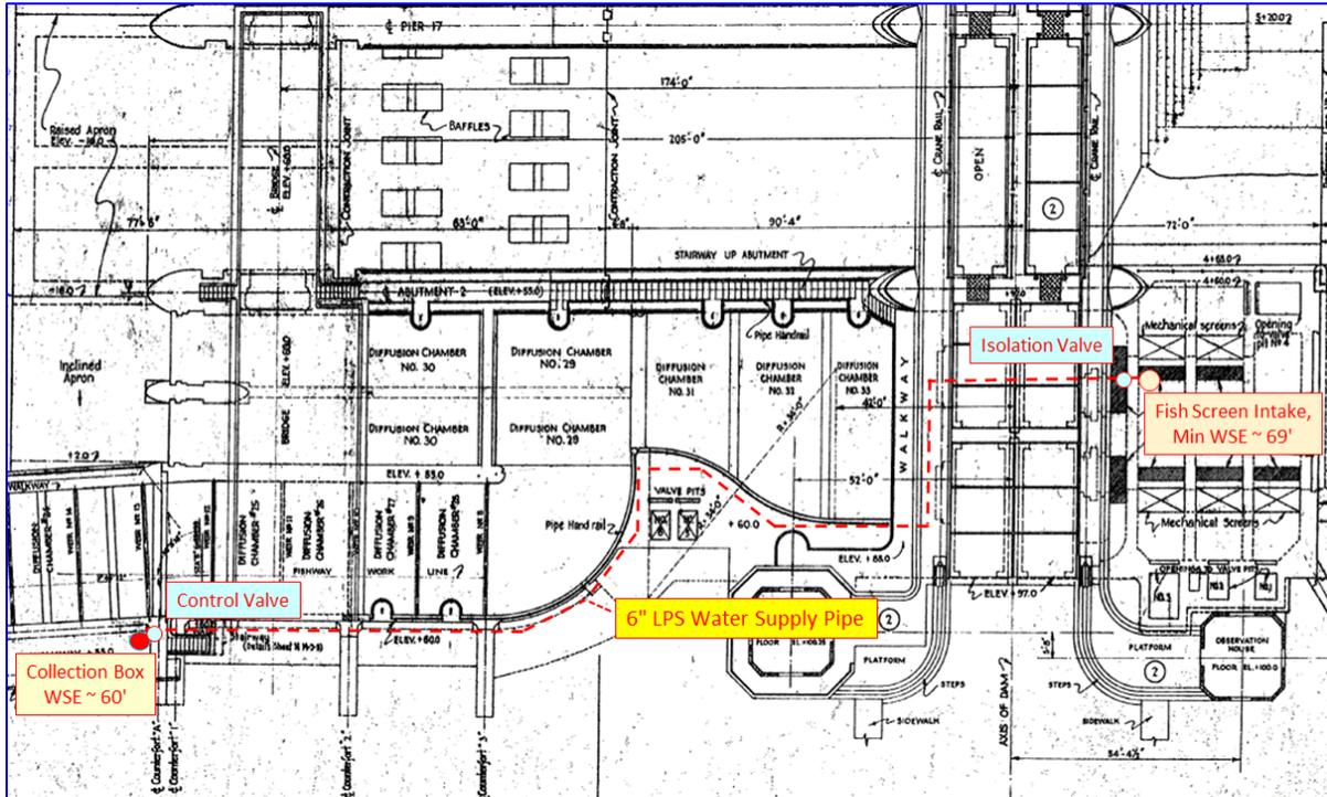
The minimum available head to the water supply system is the minimum forebay (70 feet) minus an assumed 1-foot screen loss minus collection box water surface elevation (60 feet) = 9 feet. The maximum available head is 17 feet at maximum forebay (77 feet) and neglecting screen or intake losses.
