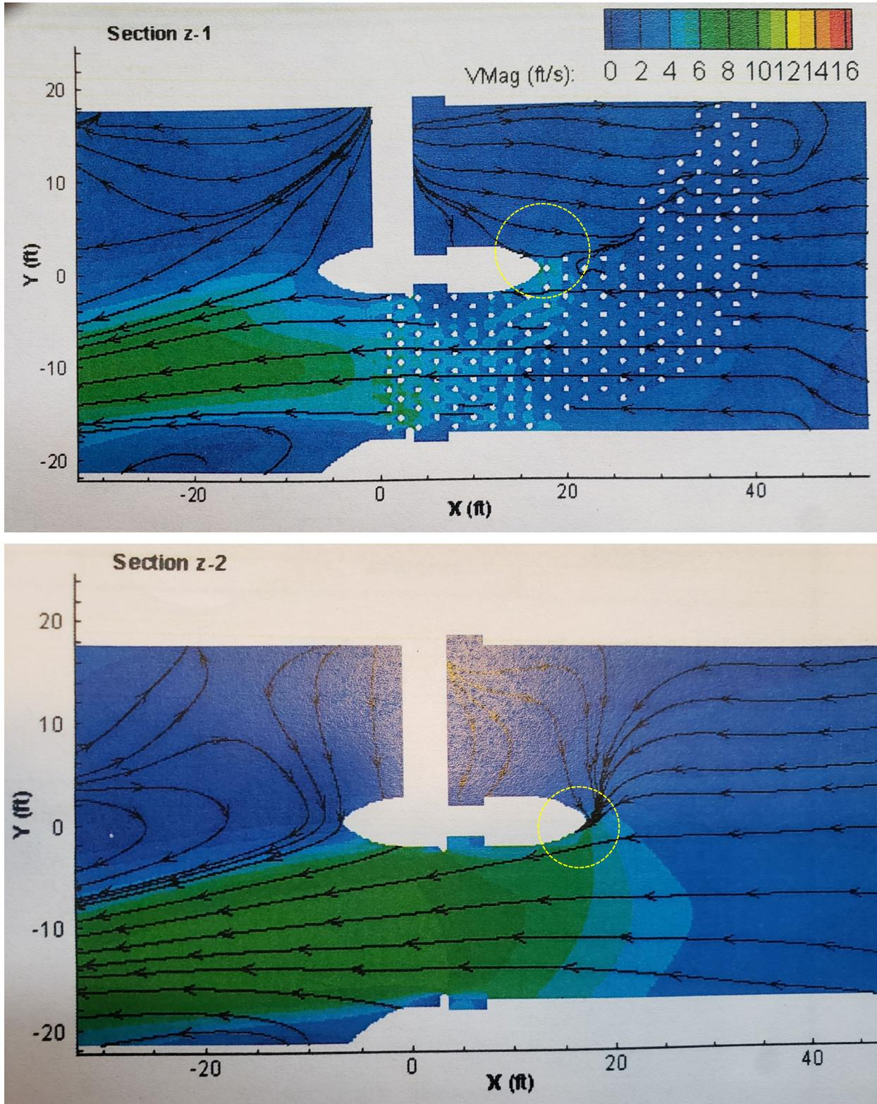
Figure 3-15. Cascade Island CFD Results (Excerpt Fig. 4-12, AECOM 2009)
