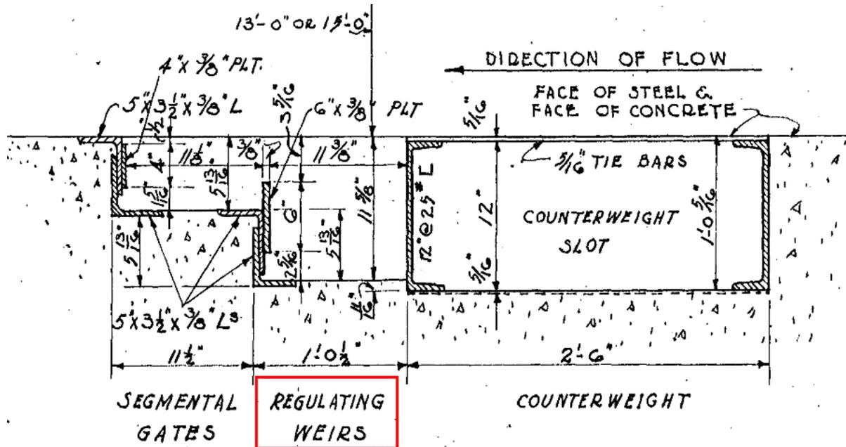
Figure 4-1: Variable Width Weir Slot shown in Red
