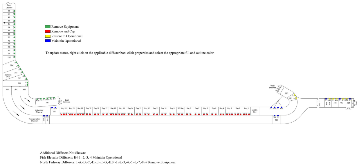
Figure 6: For TDA EFL diffuser gates, the Project has identified the diffusers that are to have moving equipment removed and remain permanently open (green), moving equipment removed and remain permanently closed (red), restored to operating condition (yellow), and remain operational (blue).
