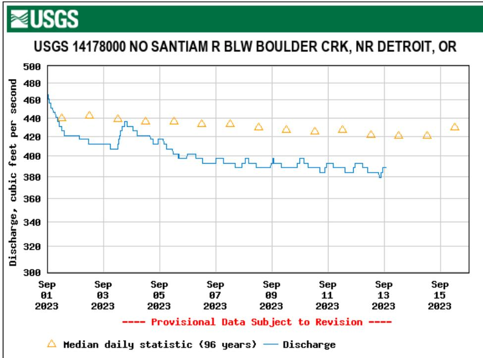
**Figure 12. Discharge (cfs); Detroit Head of Reservoir – North Santiam River**
