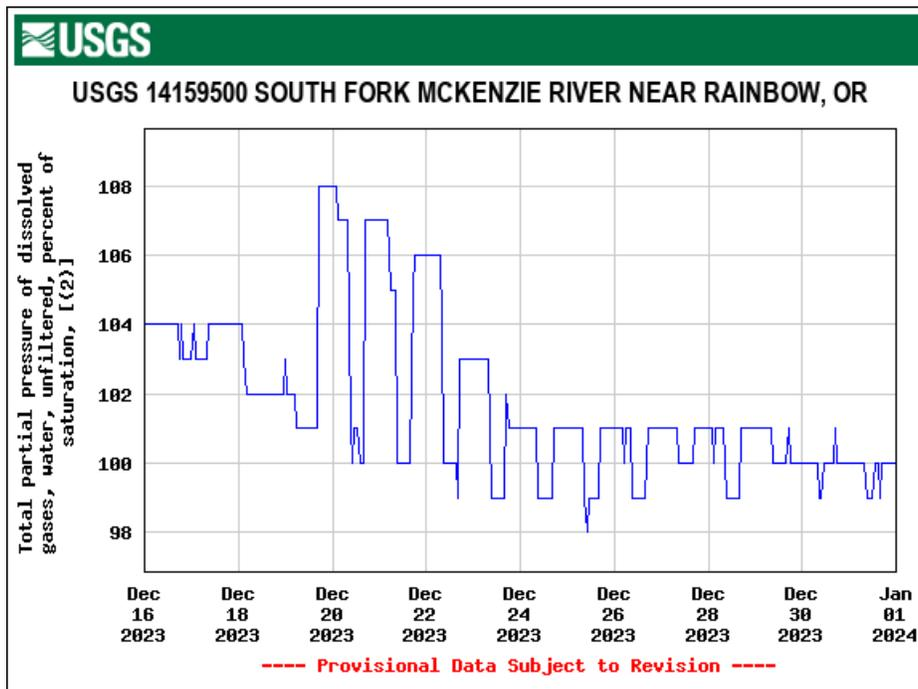
Figure 35. Total Dissolved Gas Saturation (%); below Cougar Dam, South Fork McKenzie River.
