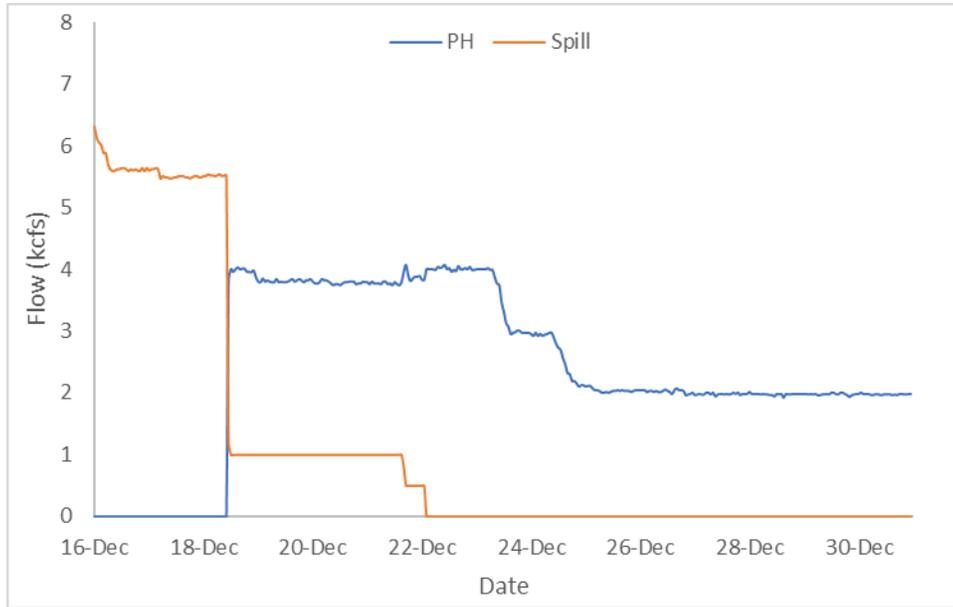
**Figure 52. Hourly Flows PWR vs. Spill (Dexter Dam).**
