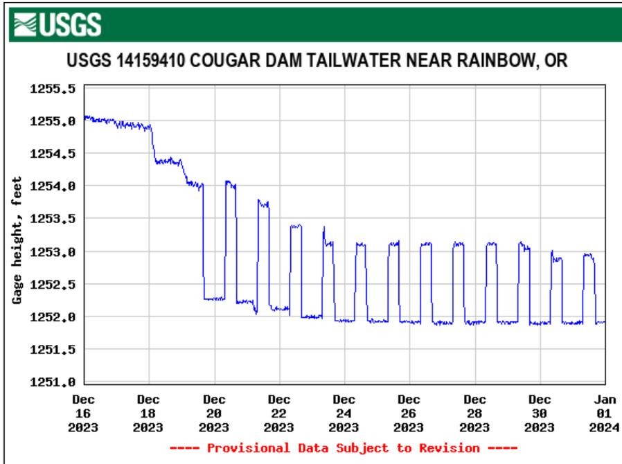
Figure 34. Gauge Height (feet); below Cougar Dam, South Fork McKenzie River.
