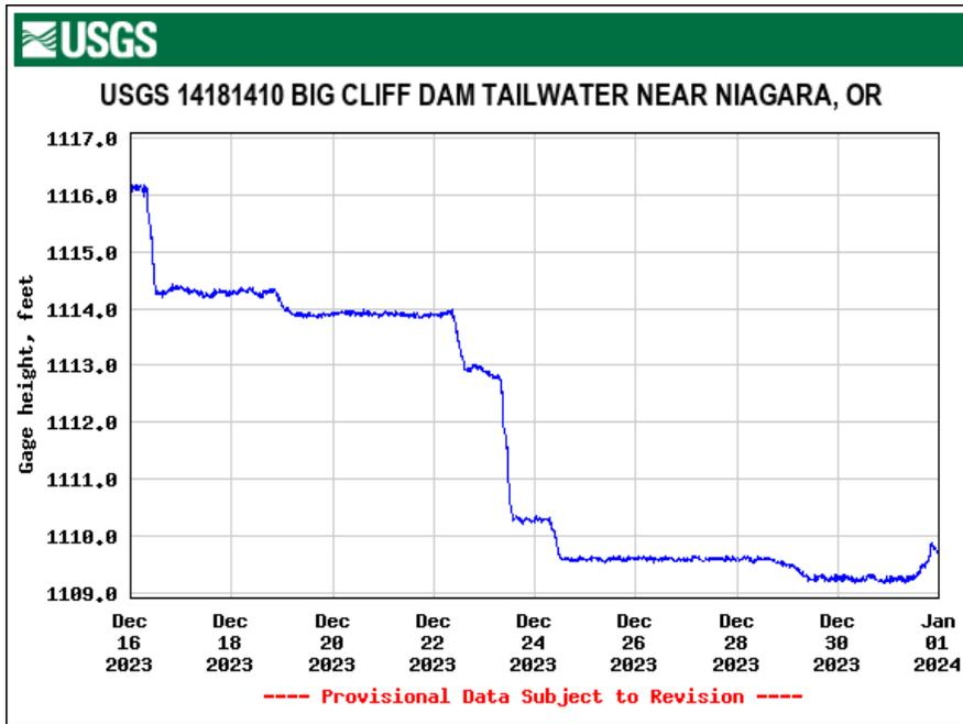
**Figure 19. Gauge height (ft); below Big Cliff Dam.**
