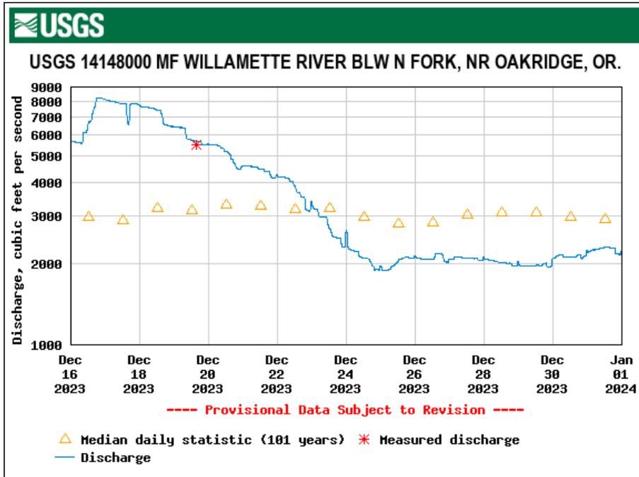
Figure 61. Discharge (cfs); above Lookout Point Reservoir, Below Oakridge, OR.
