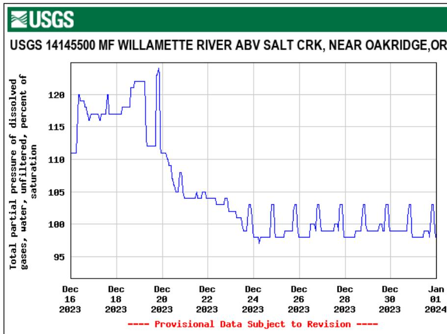
Figure 68. Total Dissolved Gas Saturation (%); below Hills Creek Dam – Middle Fork Willamette River.
