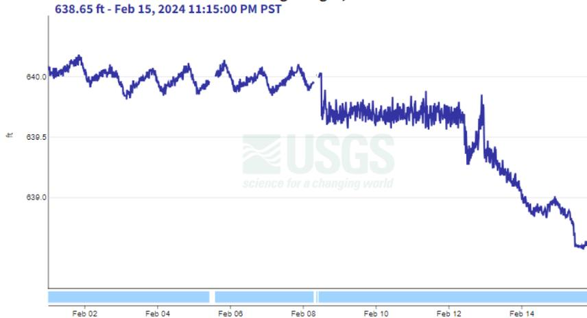
**Figure 67. Gauge Height (feet); below Dexter Dam, Middle Fork Willamette.**
