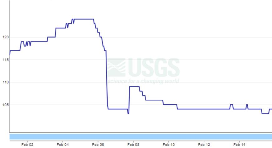
Figure 89. Total Dissolved Gas Saturation (%); below Hills Creek Dam – Middle Fork Willamette River.
