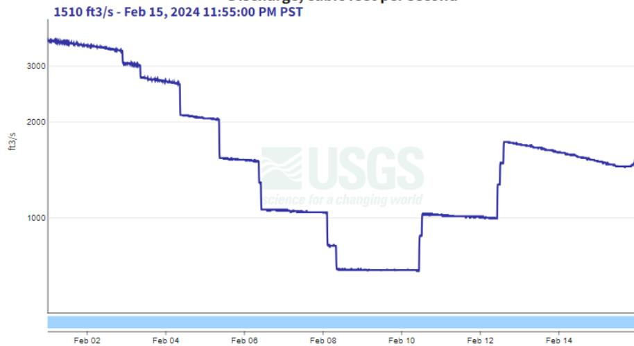
**Figure 61. Discharge (cfs); Fall Creek Below Winberry Creek, Near Fall Creek, OR**
