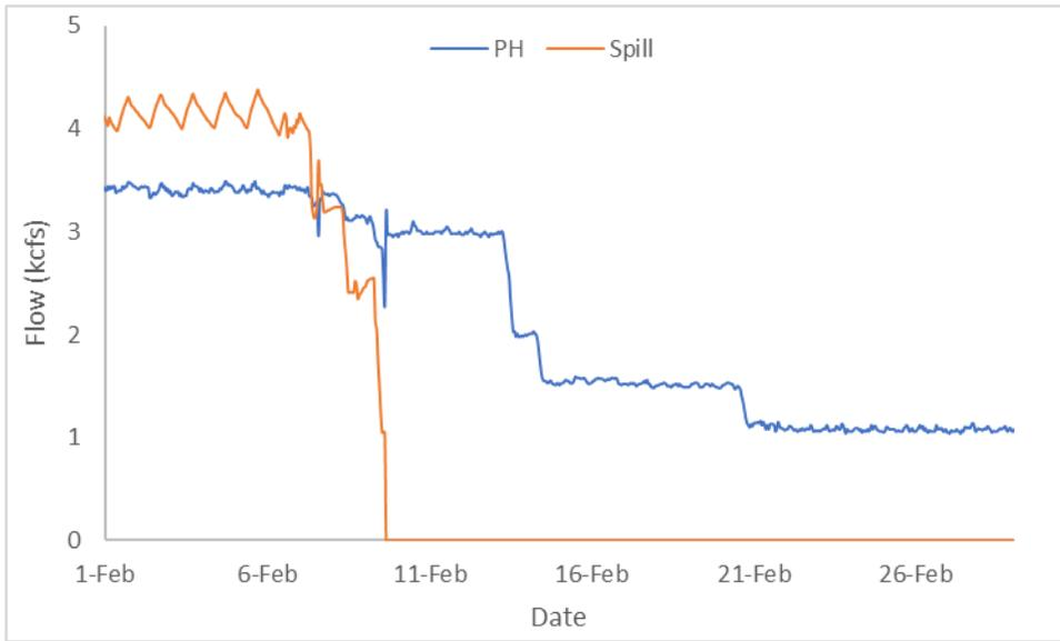
**Figure 25. Hourly Flows PWR vs. Spill (Big Cliff Dam).**
