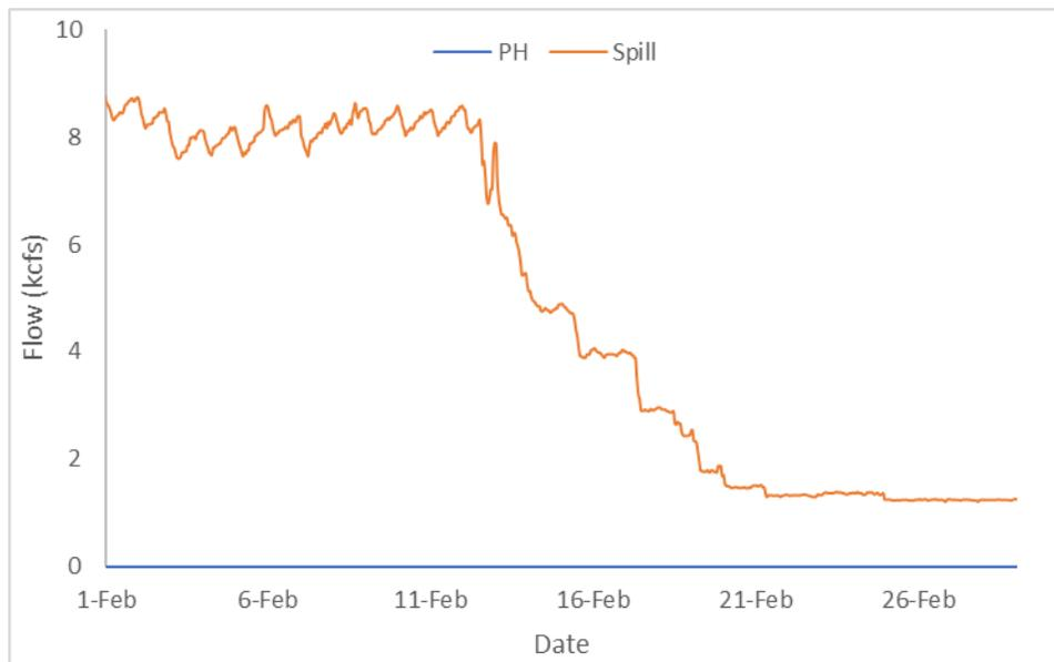
**Figure 70. Hourly Flows PWR vs. Spill (Dexter Dam).**
