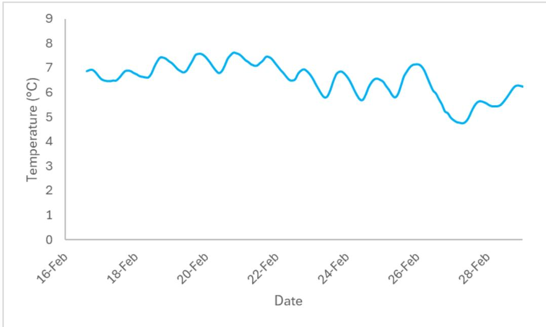
Figure 43. Temperature at RST (Foster Dam Head of Reservoir).
