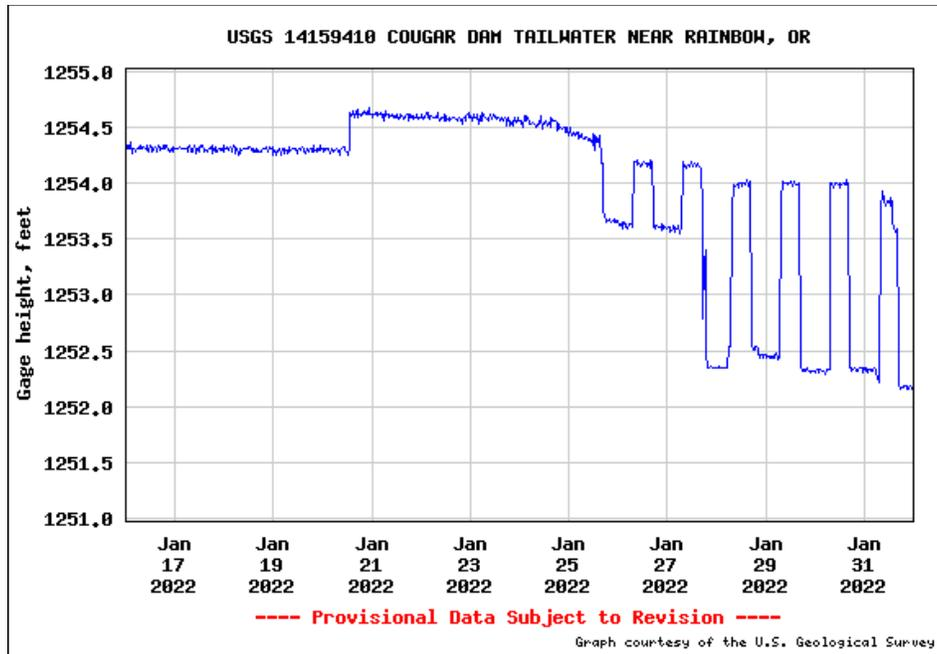
**Figure 13. Gage Height (feet); below Cougar Dam, South Fork McKenzie River**
