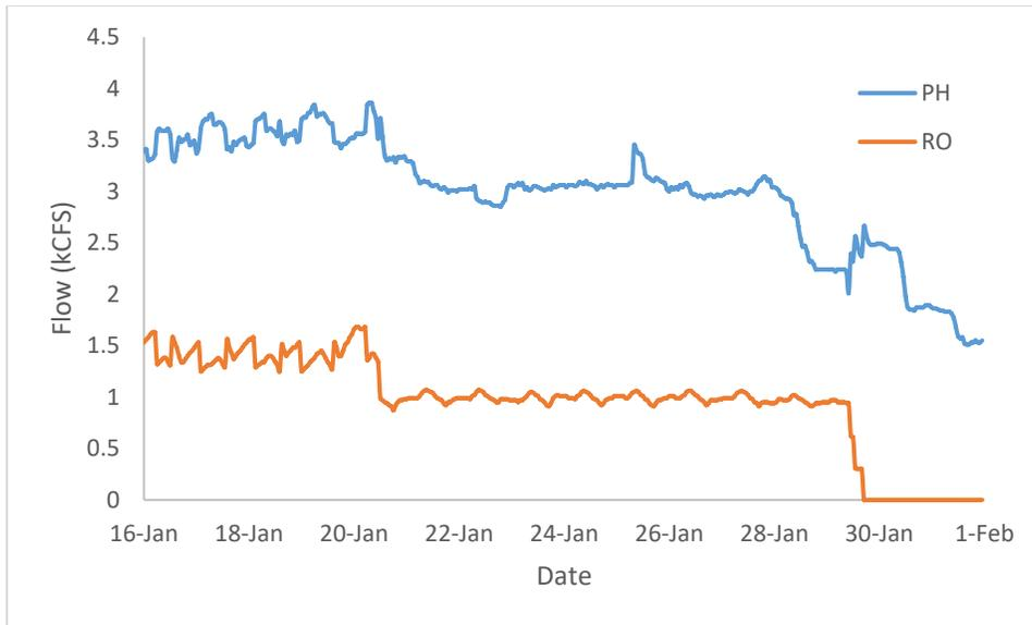
**Figure 21. Hourly Flows PWR vs. Spill (Big Cliff)**
