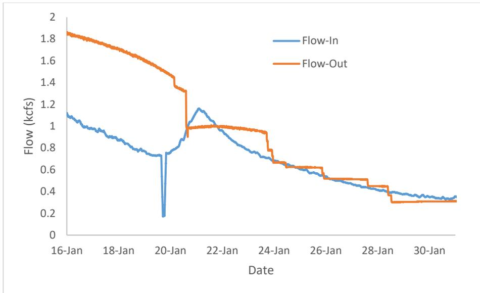
**Figure 24. Hourly Flows IN vs OUT (Fall Creek Dam)**
