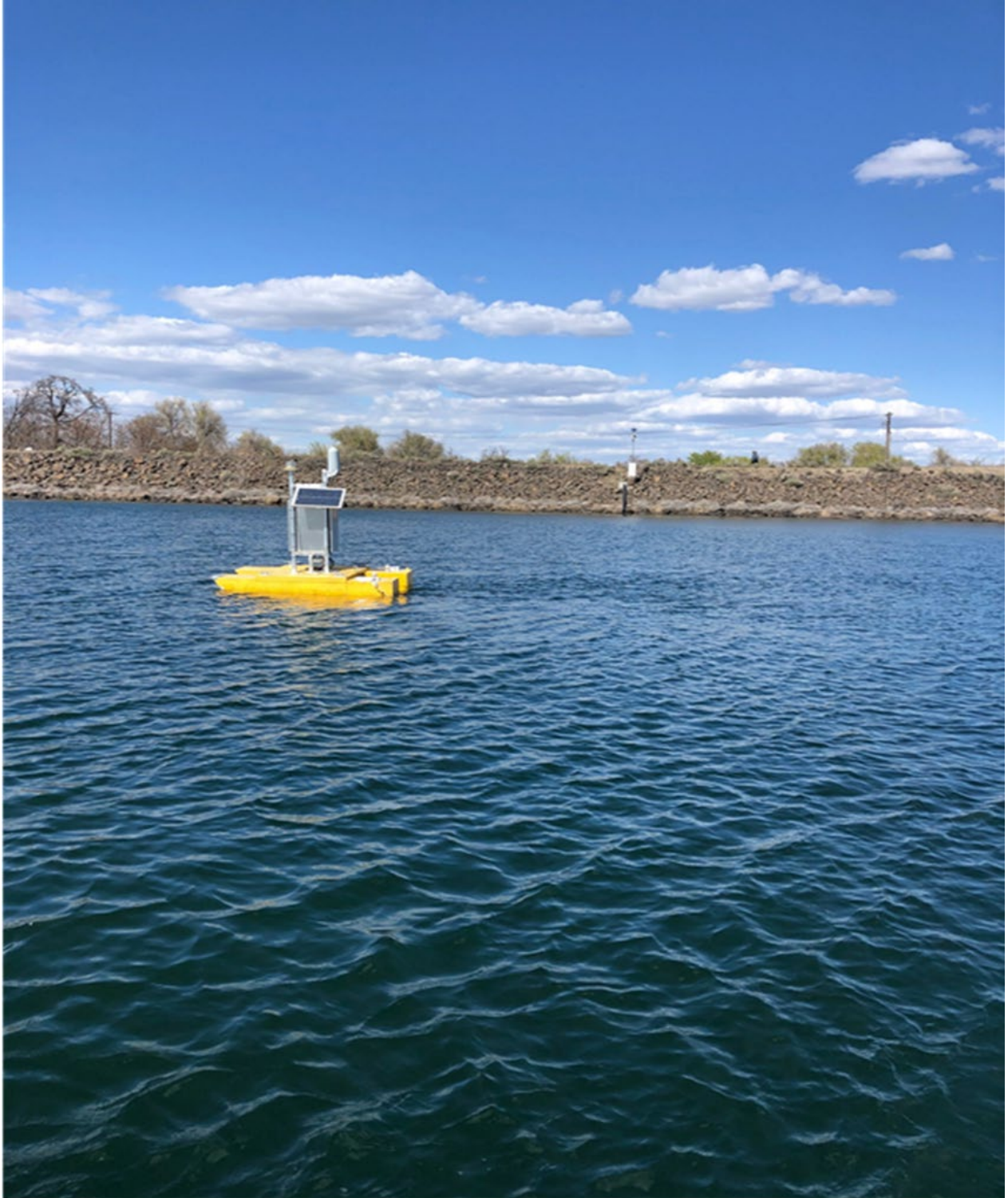
Figure F-11. Temporary PAQW TDG floating platform relative to previous onshore station.
