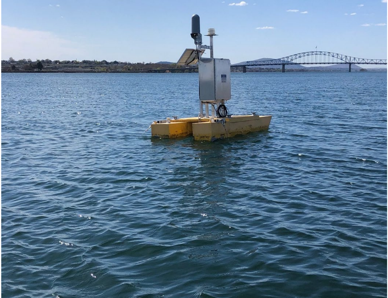
Figure F-10. Temporary PAQW TDG floating platform.
